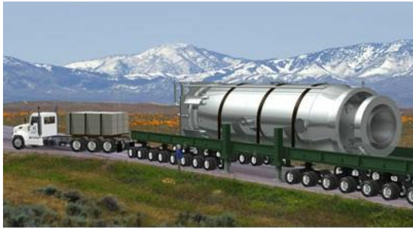
The small size of the completed NuScale power module permits component shipment via conventional large object transport such as truck, rail, and barge. Image courtesy of NuScale Power, LLC.
